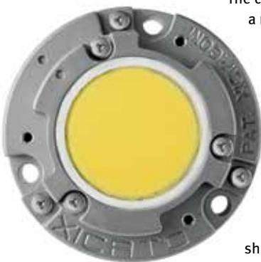
The colour temperature shift is a result of the LED ageing process, meaning the light colour of the LED changes with progressive age and use. When in use LEDs convert approx. 40% of the consumed energy into heat. The more unnecessary and „harmful“ heat is produced, the faster the colour temperature shift occurs.
