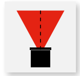
Reflector 20% scat Y10% = 2 x 22,6° Y50% = 2 x 13°
