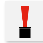
Reflector 0% scat Y10% = 2 x 6,6° Y50% = 2 x 3,6°
