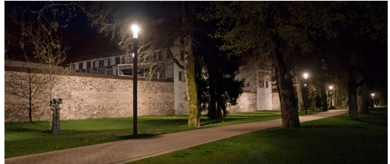
The targeted illumination of the historic wall is effected by two intermediate elements, while the top element of the CITY ELEMENTS ensures the homogeneous illumination of the footpath and cycle way.
